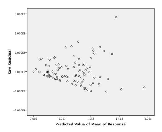
Figure 7. Plot of homoscedasticity of residuals vs. the predicted values for original data
